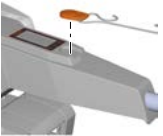
Fig. 57: Magnetic kill switch
